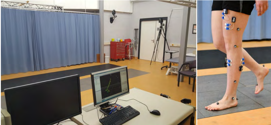
Figure 1.3: A typical laboratory-based optical motion capture system for human movement analysis (Left). A subject with reflective markers strapped onto the body for movement analysis (Right)
