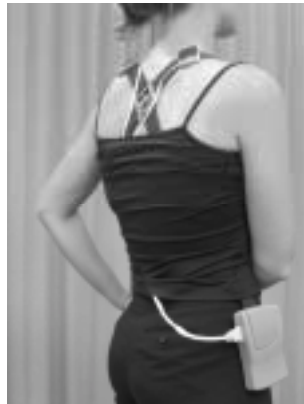
Picture 1.1: Myofeedback device consisting of a harness with dry surface electrodes and a sEMG storage and processing unit
