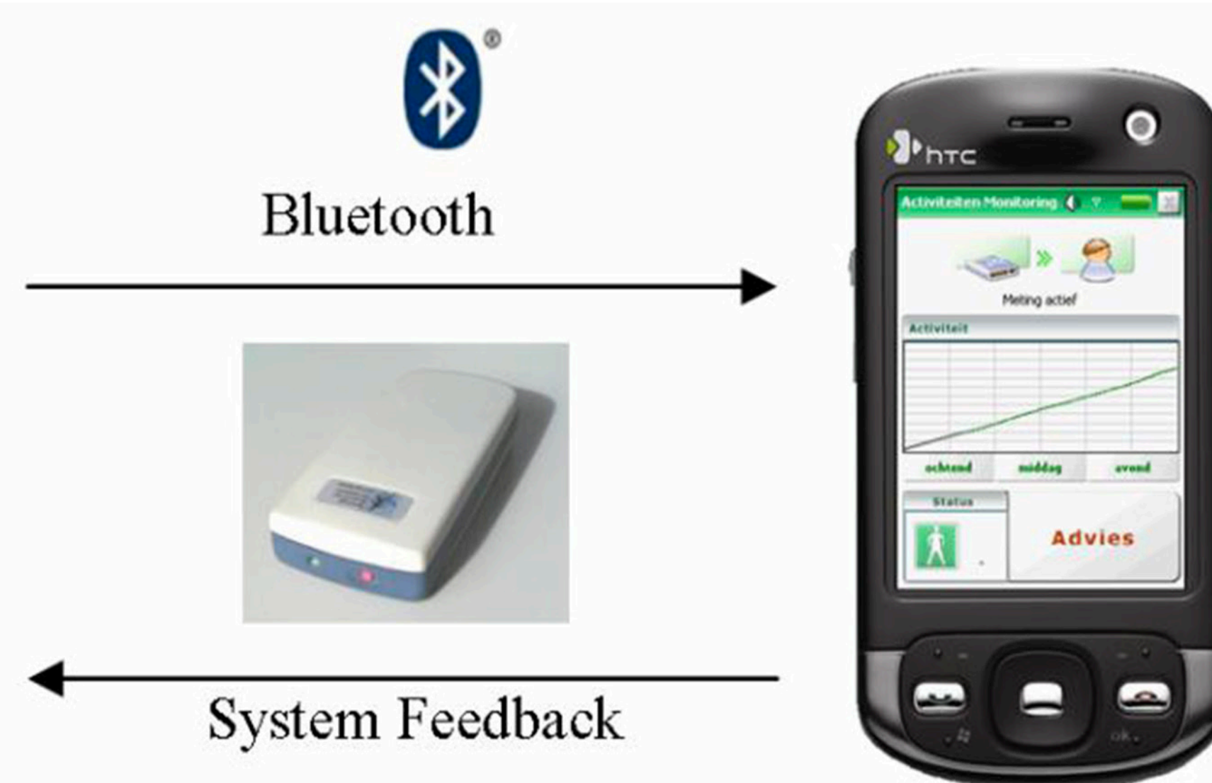
Figure 1: The telemedicine feedback intervention: triaxial accelerometer for measuring activity (in counts per minute) and PDA for providing feedback to the patient.
