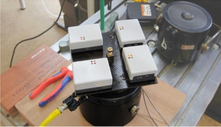
Figure 6. Setup of the sensors on the mechanical oscillator. Four ProMove2 sensors were securely fastened to a mechanical oscillator (Vibration Exciter, type 4809, Brüel & Kjær).
