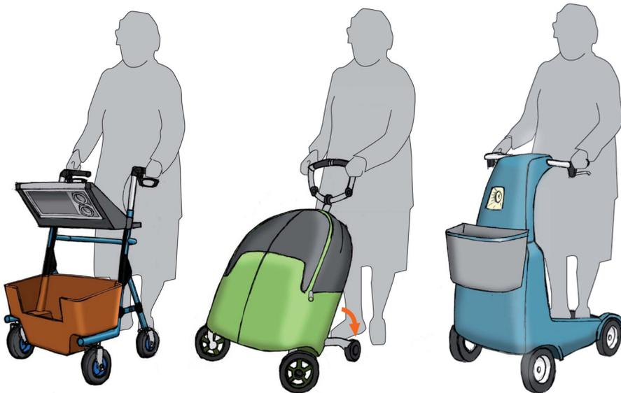
Figure 24 The three selected designs. Left: the multifunctional wheeled walker; Middle: the grow-along grocery bag; and Right: the electric wheeled walker. For more details see Appendix 2.
